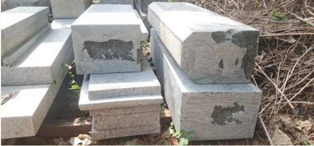
Carved black granite elements — column caps and pillar bases being prepared in Kerala.
